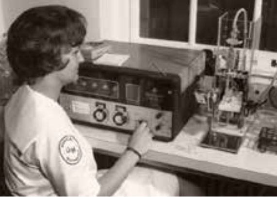
A lab technician uses a coulter counter to analyze blood samples; circa 1970s.
